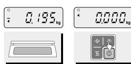
Remove container and commodity, then the display will show the weight of the container with "-" symbol.
